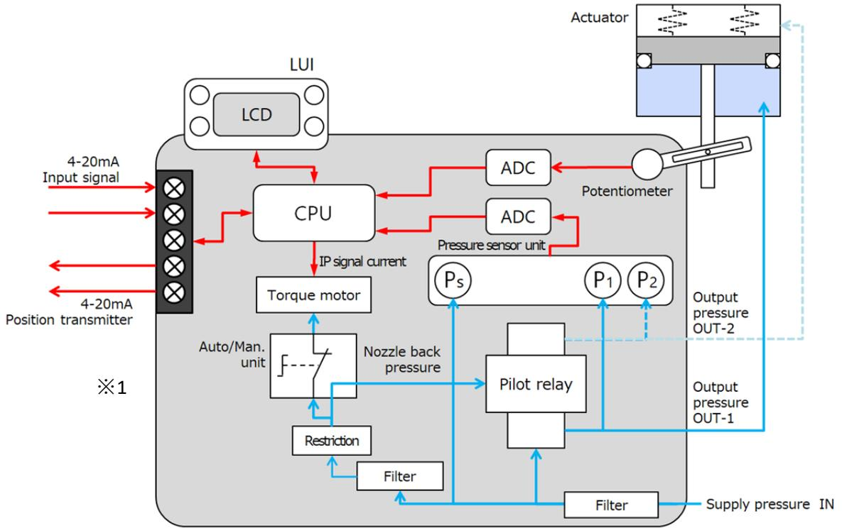
Figure 1.3.2a Principle of operation
