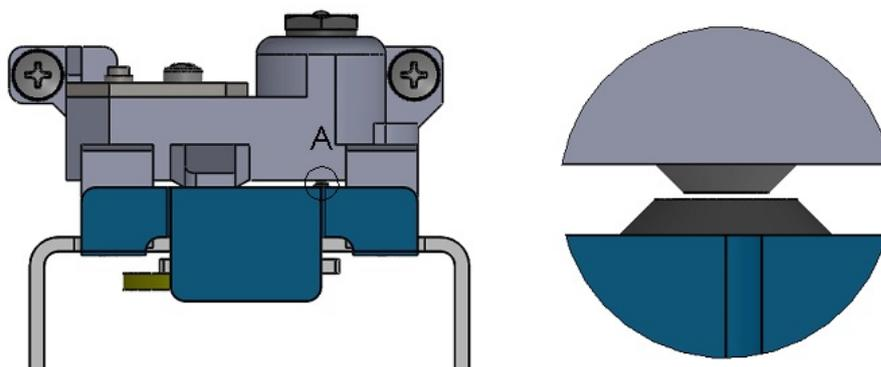
Figure 5.4.3 Cleaning site of nozzle flapper
