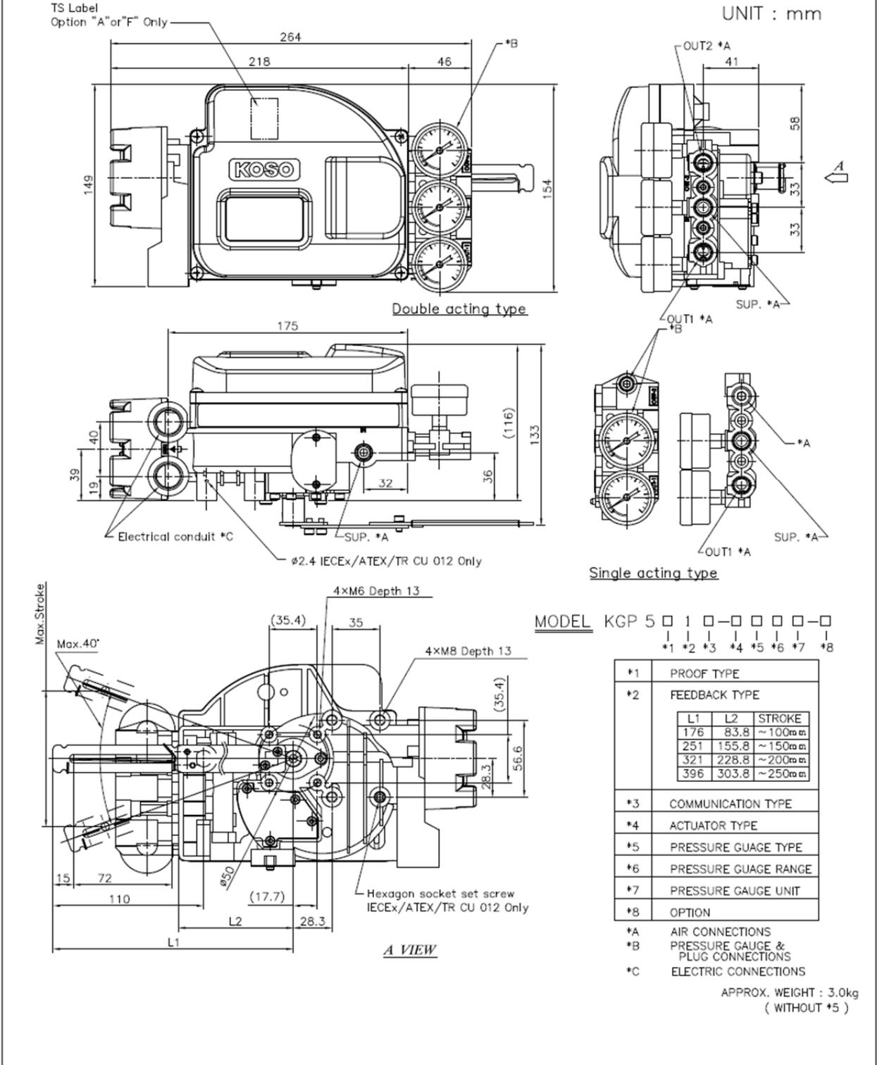
Fig. 11b Linear motion long stroke type
