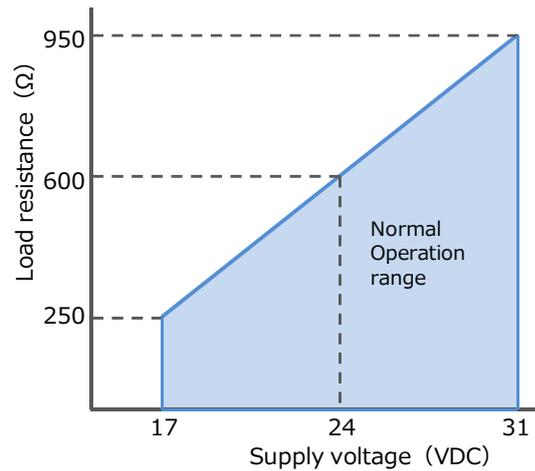
Figure 2.6f Load resistance to supply voltage relationship via the connection of position transmitter
