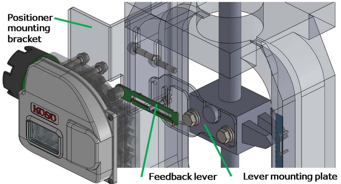
Figure 2.2a Example of mounting to linear motion actuator
