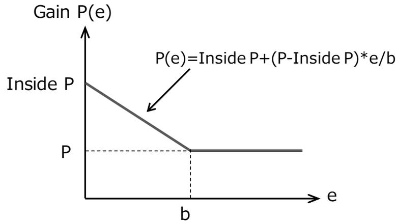
Figure 4.5.2. Gain switching (Example of proportional gain)
